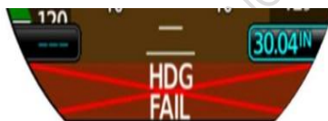
Figure 6- Bottom of the ADI when HDG failed (no GPS)
