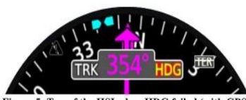
Figure 5- Top of the HSI when HDG failed (with GPS)
