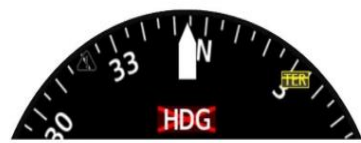
Figure 7- Top of the HSI when HDG failed (no GPS)
